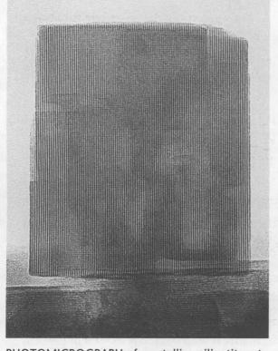
PHOTOMICROGRAPH of crystalline silicotitanate material shows the cage-like molecular structure that allows the material to capture ions small enough to reach vacant bonding sites within the structure, such as cesium, and reject slightly larger ions, such as sodium.
